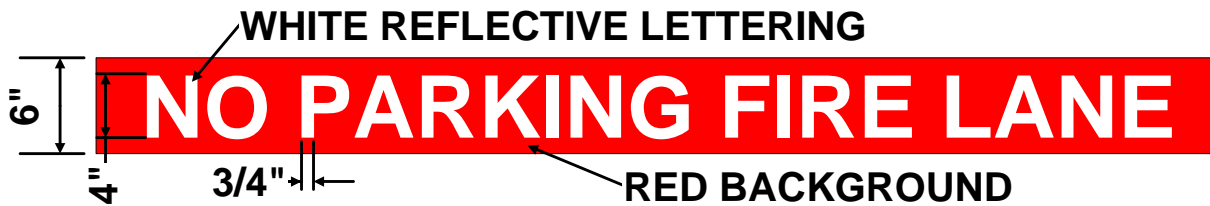
FIGURE D103.7 FIRE LANE STRIPING
